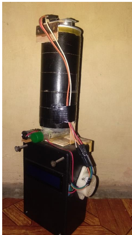
Figure 8. Installation of Feeder Equipment in the Aquarium
