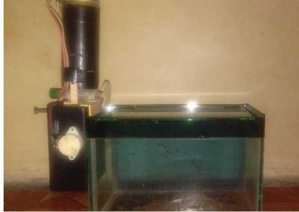
Figure 7. Installation of Feeder Equipment in the Aquarium
